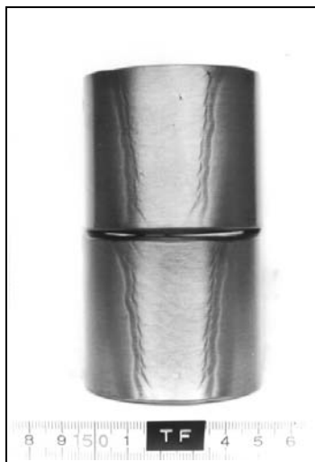
Fig. 6.4 — Side bend specimens after test
