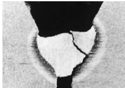
(F) Root crack
