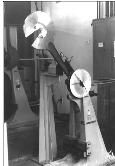
Fig. 6.7 — A Charpy impact test machine
