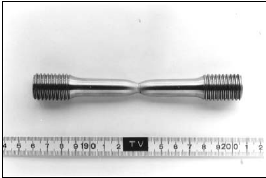
Fig. 6.2 — A Tension test specimen after test
