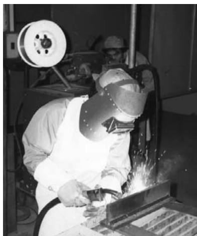
Fig. 4.26 — Typical protective clothing in gas metal arc welding
